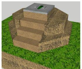
Make a sand envelope around sides and bottom of pit/rings
